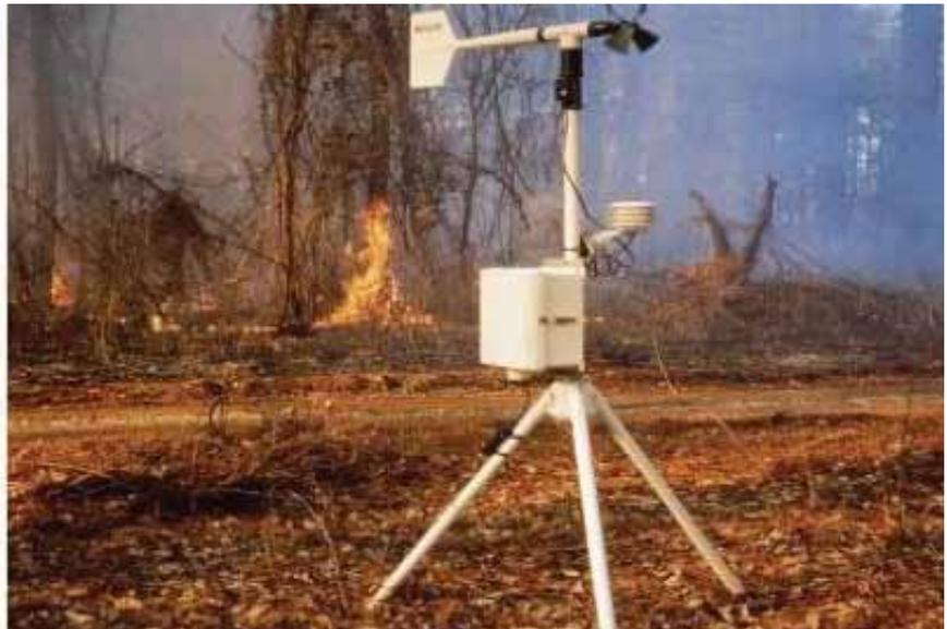
*Left: An AWS system used for determining the microclimate during a controlled fire (source: CSI). Right: A 12-plate radiation shield for air temperature measurement (also referred to as a 12-plate Gill shield) (Source: MJS).*
